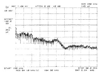
**TEST RESULTS:** Both lines were observed. The measurements indicate that the unit DOES appear to meet the FCC requirements for this class of equipment.
