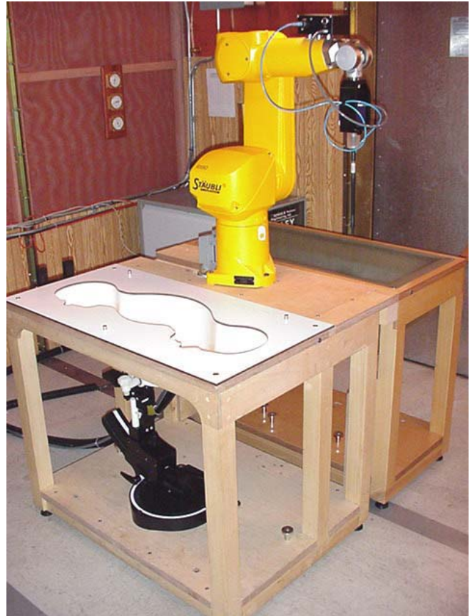
DASY4 SAR Measurement System with SAM phantom
