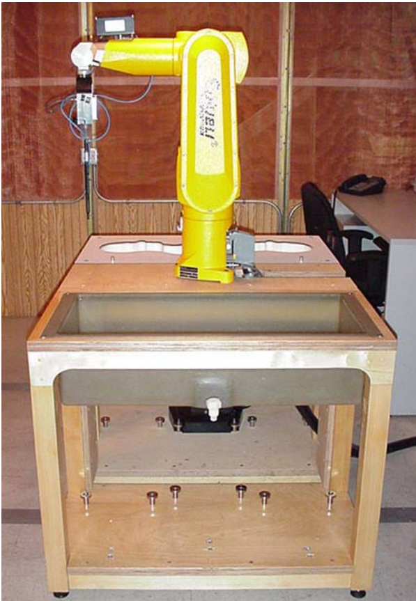
DASY4 SAR Measurement System with planar phantom
