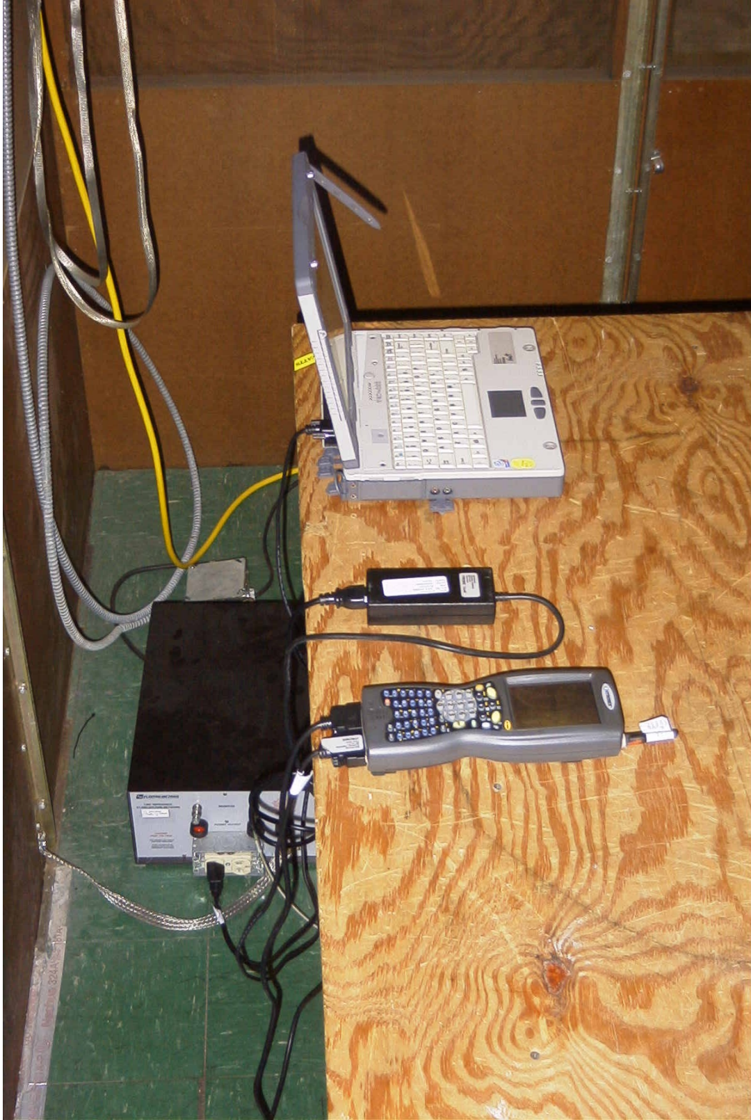
POWER LINE CONDUCTED SIDE TEST SET UP PHOTOGRAPH
