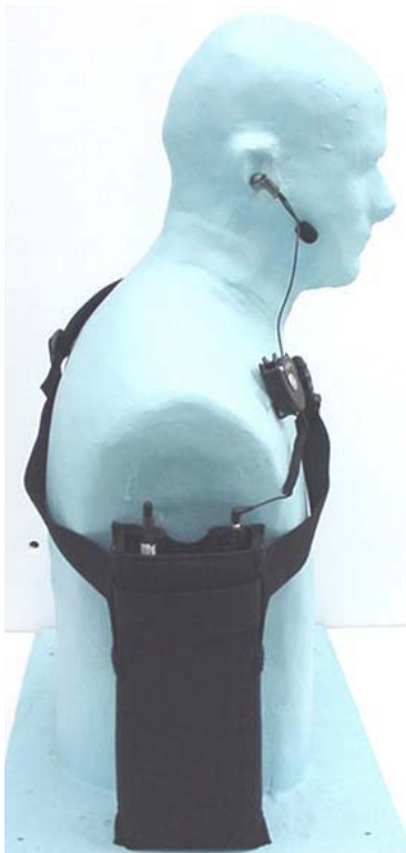
Front Side of DUT facing body - worst-case antenna configuration in relation to right arm
