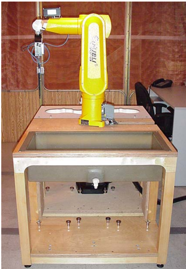
DASY4 SAR Measurement System with planar phantom
