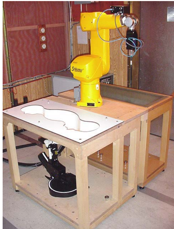
DASY4 SAR Measurement System with SAM phantom
