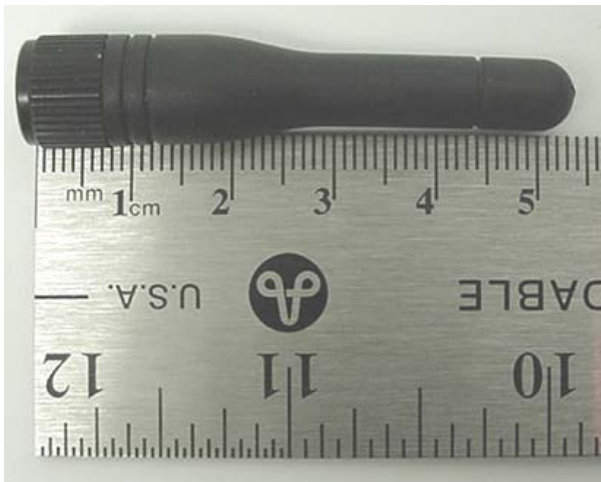
Dual-Band CDMA Antenna - 1/4 wave Helix
