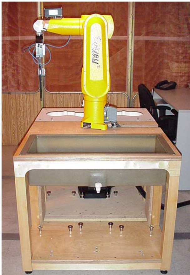
DASY4 SAR Measurement System with planar phantom
