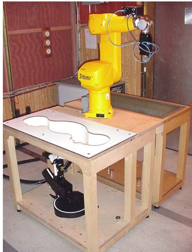
DASY4 SAR Measurement System with SAM phantom
