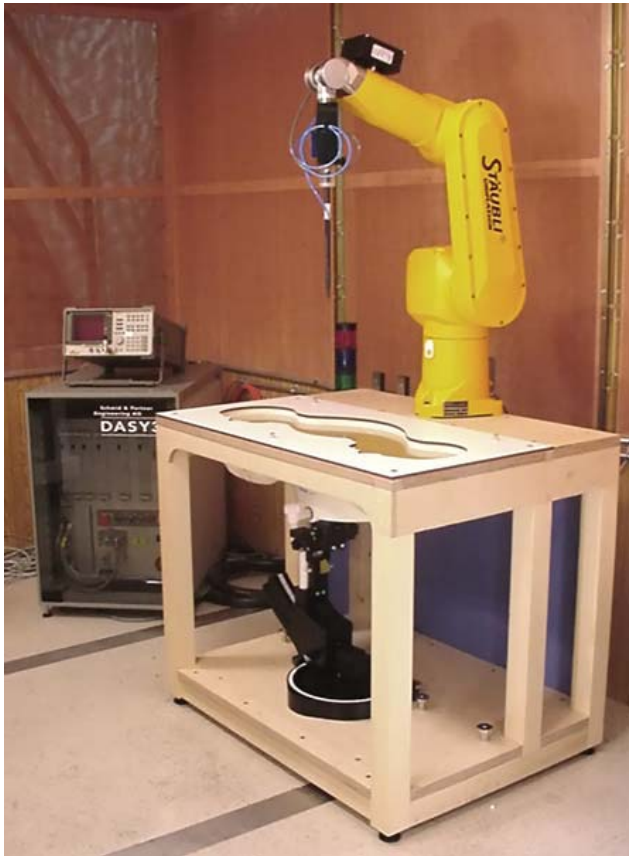
DASY3 SAR Measurement System with SAM phantom
