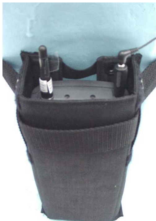
Front Side of DUT facing body - worst-case antenna configuration relative to right arm
