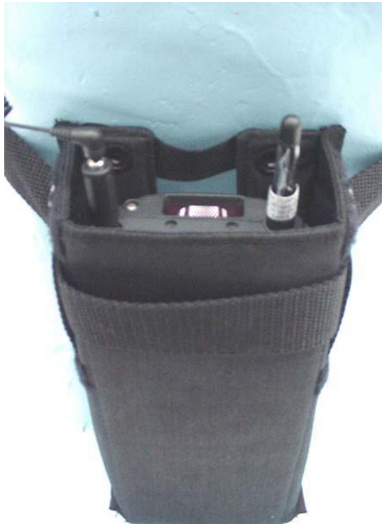
Back Side of DUT facing body - worst-case antenna configuration relative to left arm
