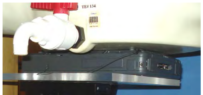
Bottom Side of DUT touching SAM phantom (planar section) – WLAN Main Antenna
