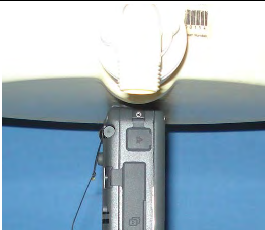
(“90° Portrait”) Adjacent Edge of DUT touching SAM phantom (planar section) – WLAN Main Antenna
