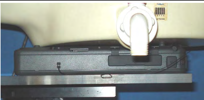
Bottom Side of DUT touching SAM phantom (planar section) – WLAN Main Antenna
