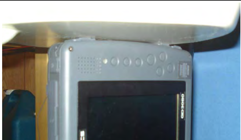
(“90° Portrait”) Adjacent Edge of DUT touching SAM phantom (planar section) – WLAN Main Antenna
