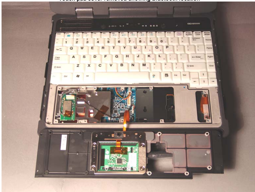
Touch pad cover removed showing Bluetooth location
