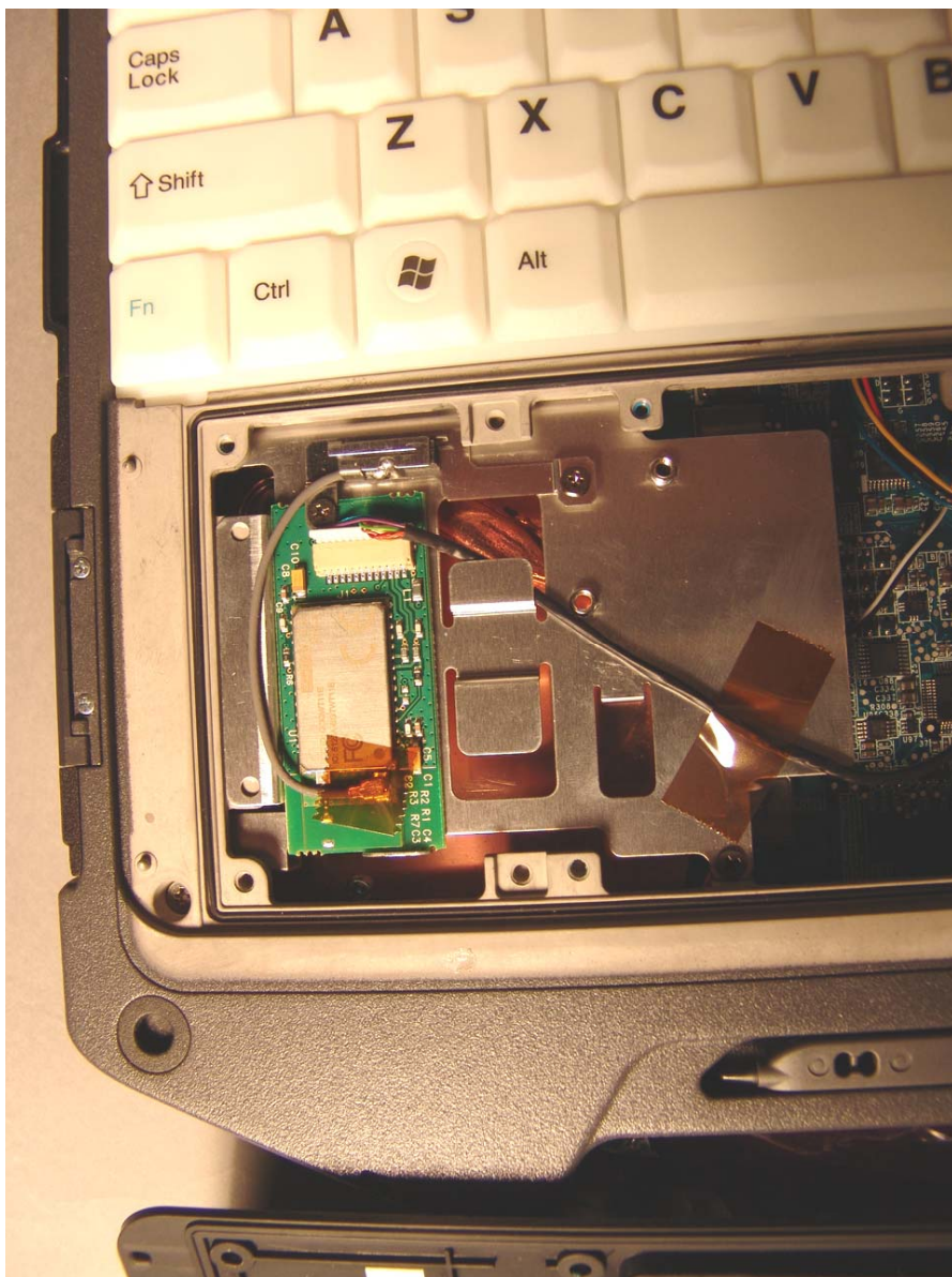
Close Up of Bluetooth Module and Antenna Location within the GD8000
