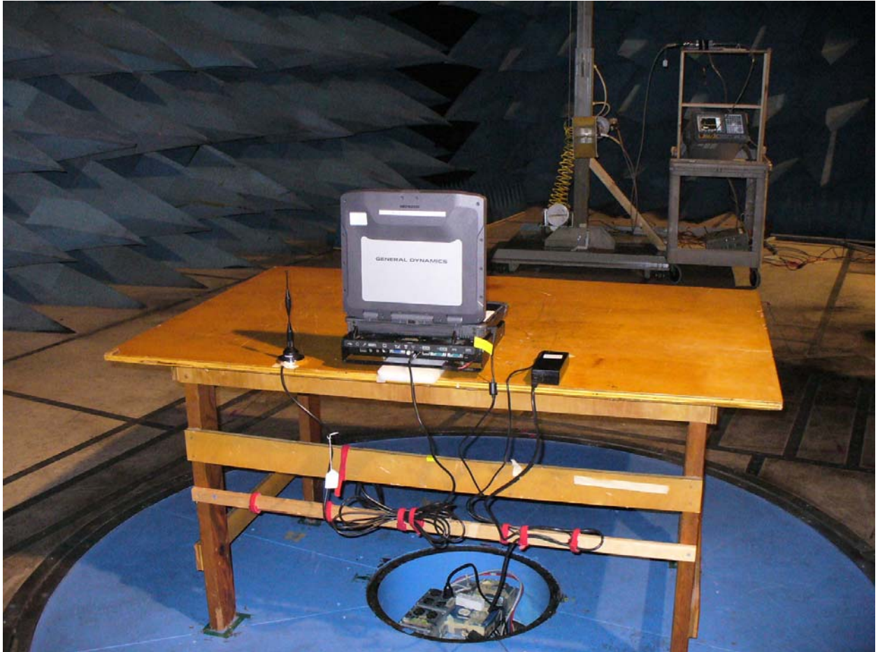
Figure 2: Radiated Emissions with Host GD8200, External Antenna – Back View
