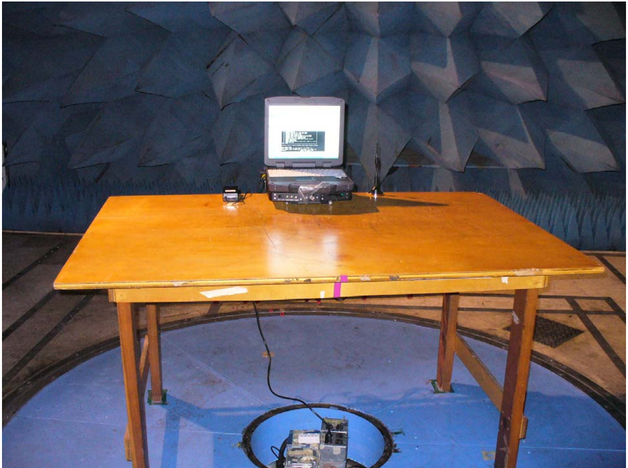
Figure 1: Radiated Emissions with Host GD8200, External Antenna– Front View
