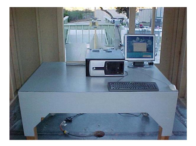
Radiated Emissions Measurement (Front View) Setup
