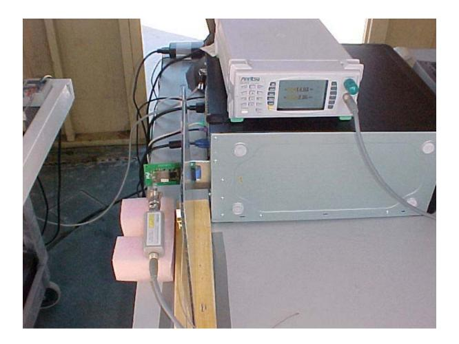
Maximum Peak Output Power Measurement Setup
