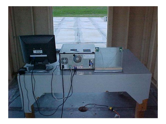
Radiated Emissions Measurement (Rear View) Setup
