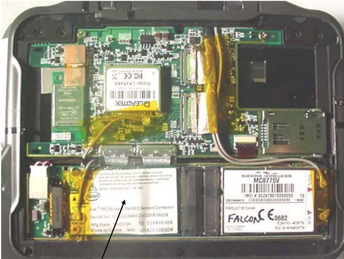
Intel 3945ABG 802.11abg WLAN Mini-PCI Express Card installed in DUT
