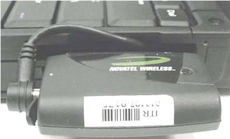
Dual-Band CDMA/EV-DO Card installed in IX600 Rugged Laptop PC PCMCIA Slot
