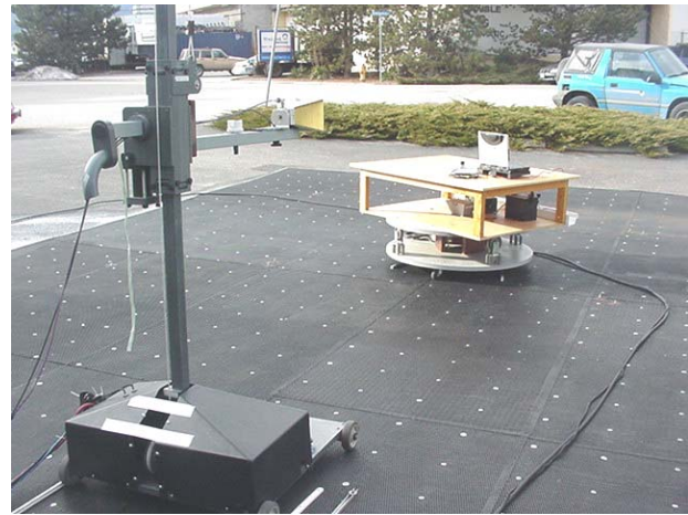
Photograph B.8-4 - Horn Receive Antenna with DUT Vehicle-Mount Antenna Configuration
