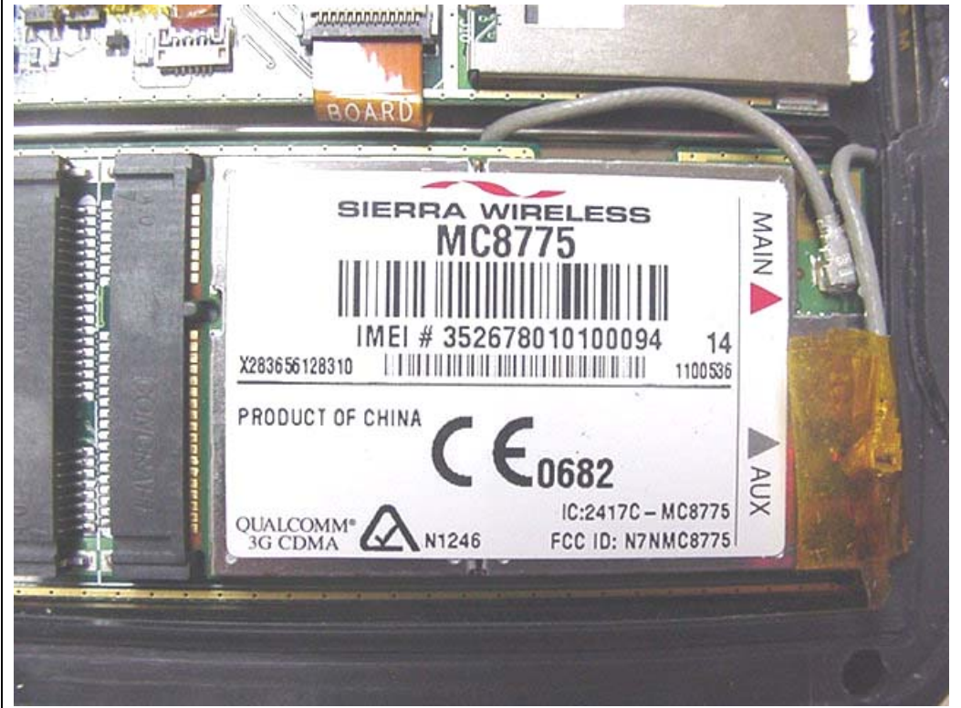
IX-MC8775 GPRS/EDGE/WCDMA Mini-PCI Express Card installed in IX750 PC
