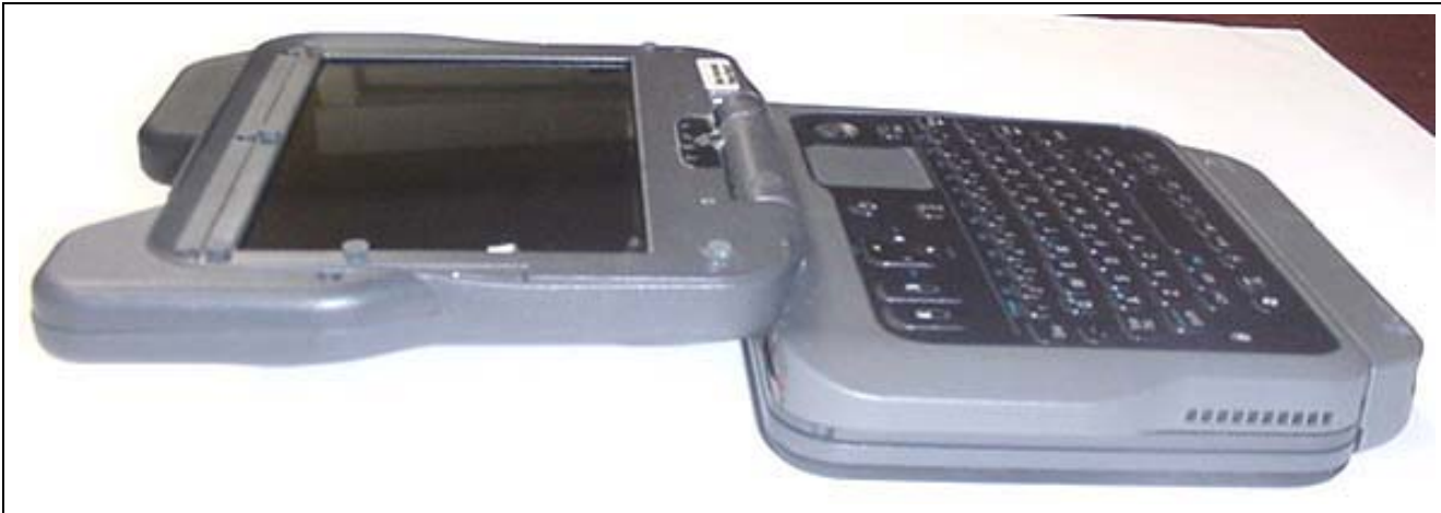
Left Side of IX750 PC with Standard Capacity Lithium-ion Battery - LCD Display Fully Extended
