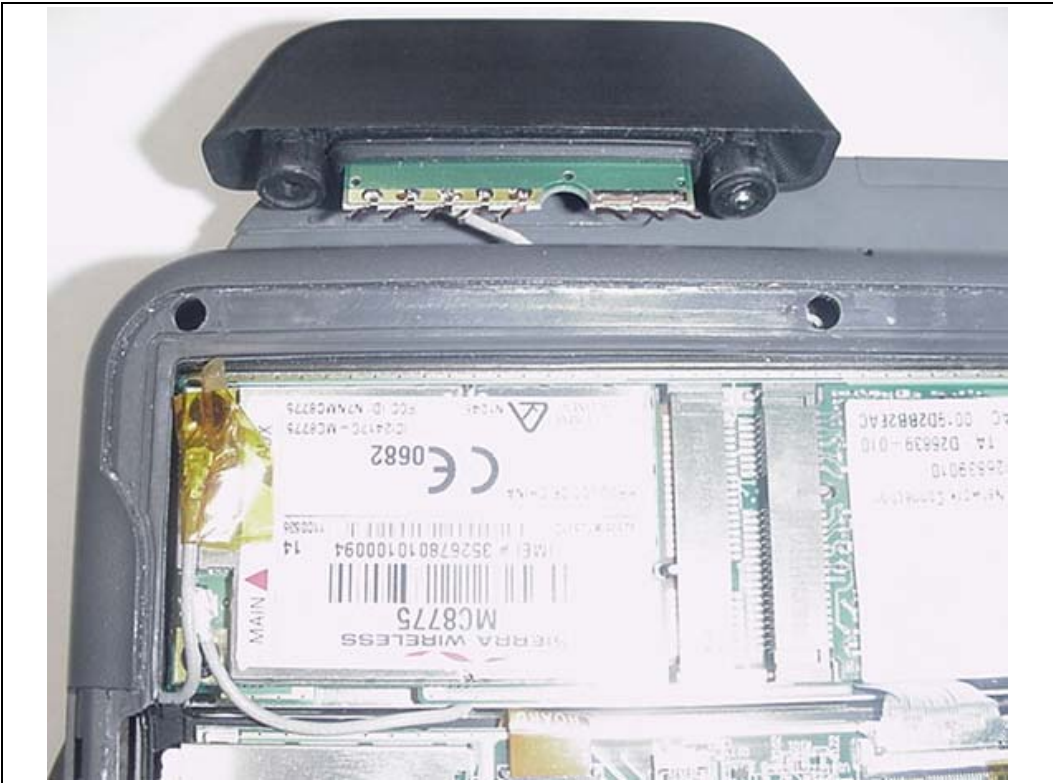
IX-MC8775 GPRS/EDGE/WCDMA Mini-PCI Express Card and Antenna installed in IX750 PC
