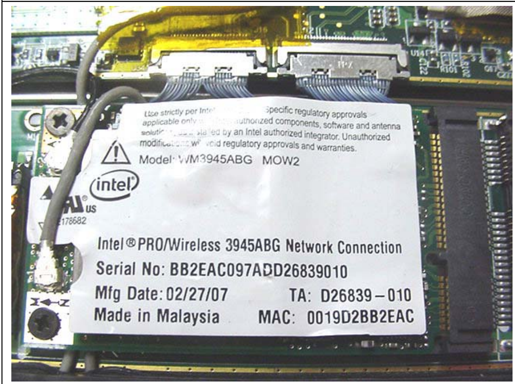
Co-located WLAN Mini-PCI Express Card Model: IX-WL3945
