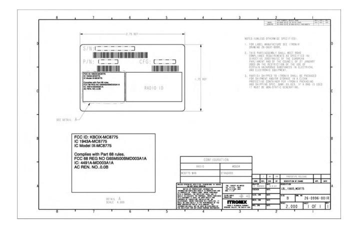
Note: Part 15.19 Label Information, IC / FCC ID label location on the IX605, and Co-Located FCC/IC Identifier labels for the KBCIX-MC8775 and KBCIX-4965AGN and KBCIX-BR-51 are located on the following pages.
