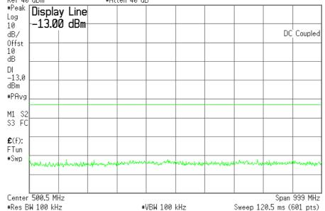
Plot 6.4.47) Out of Band Emissions at Antenna Terminals
