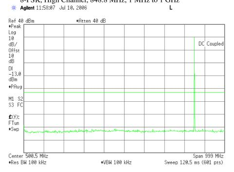
Plot 6.4.17) Out of Band Emissions at Antenna Terminals
