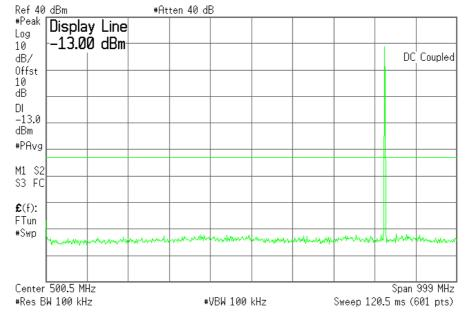
Plot 6.4.11) Out of Band Emissions at Antenna Terminals
