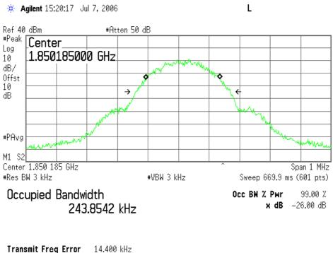
**5.3.8) GMSK Occupied Bandwidth**, PCS Middle channel, 1880.0 MHz, 99% bandwidth
