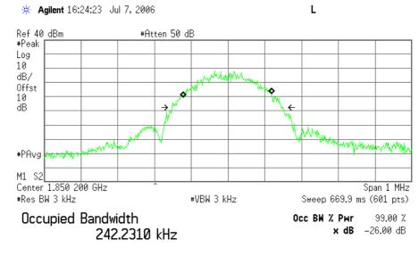
**Transmit Freg Error** -1.983 kHz Occupied Bandwidth
