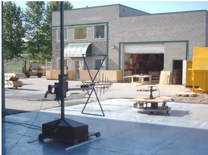
Photograph B.8-3 - Dipole Substitution Setup
