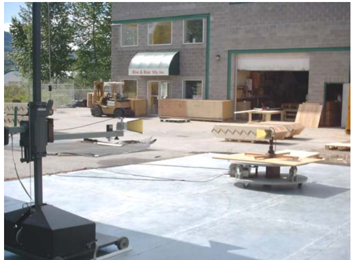
Photograph B.8-4 - Horn Substitution Setup
