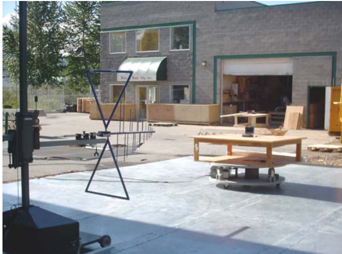
Photograph B.8-3 - Dipole Substitution Setup
