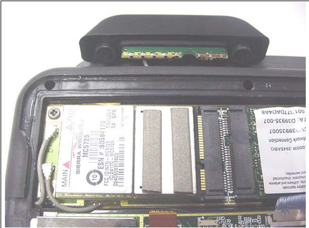
IX-MC5725 Dual-Band CDMA/EVDO Mini-PCI Express Card and Antenna installed in IX750 PC
