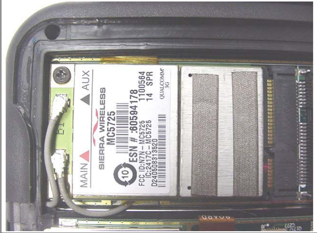
IX-MC5725 Dual-Band CDMA/EVDO Mini-PCI Express Card installed in IX750 PC
