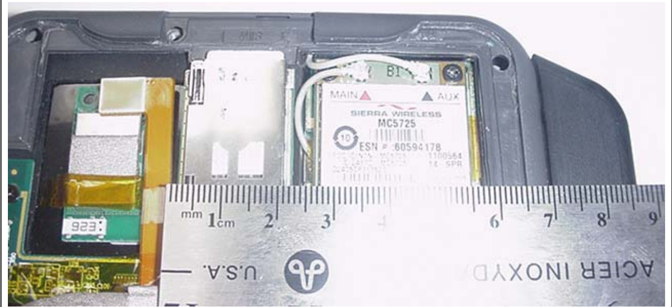
Spacing between Co-Transmitting Bluetooth Antenna and IX-MC5725 Antenna (> 5.0 cm)
