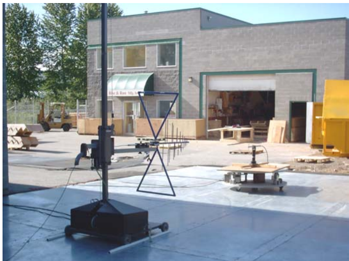
Photograph B.8-3 - Dipole Substitution Setup
