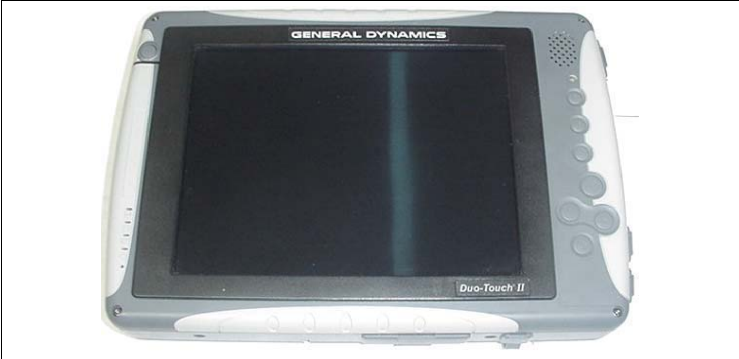
General Dynamics Itronix Corporation Ruggedized Tablet PC Model: IX350 - "0 Degrees Landscape" LCD Display Orientation
