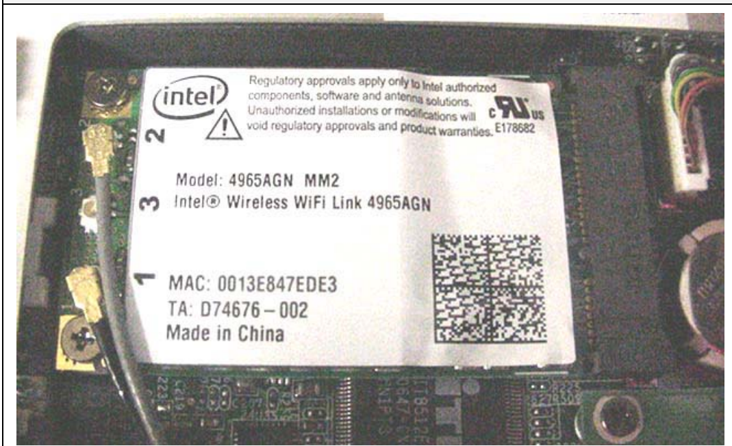
IX-4965AGN WLAN Mini-PCI Express Card
