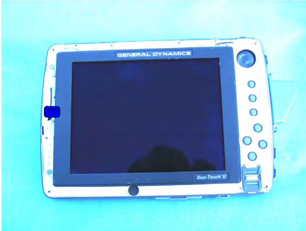
Bluetooth Antenna Left Side Center on IX350 Above, Shown Below
