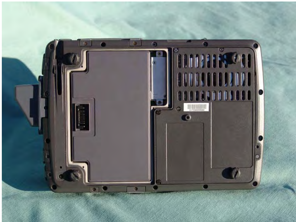
Bottom View Battery Cover removed, WLAN and Bluetooth Radios are located under battery
