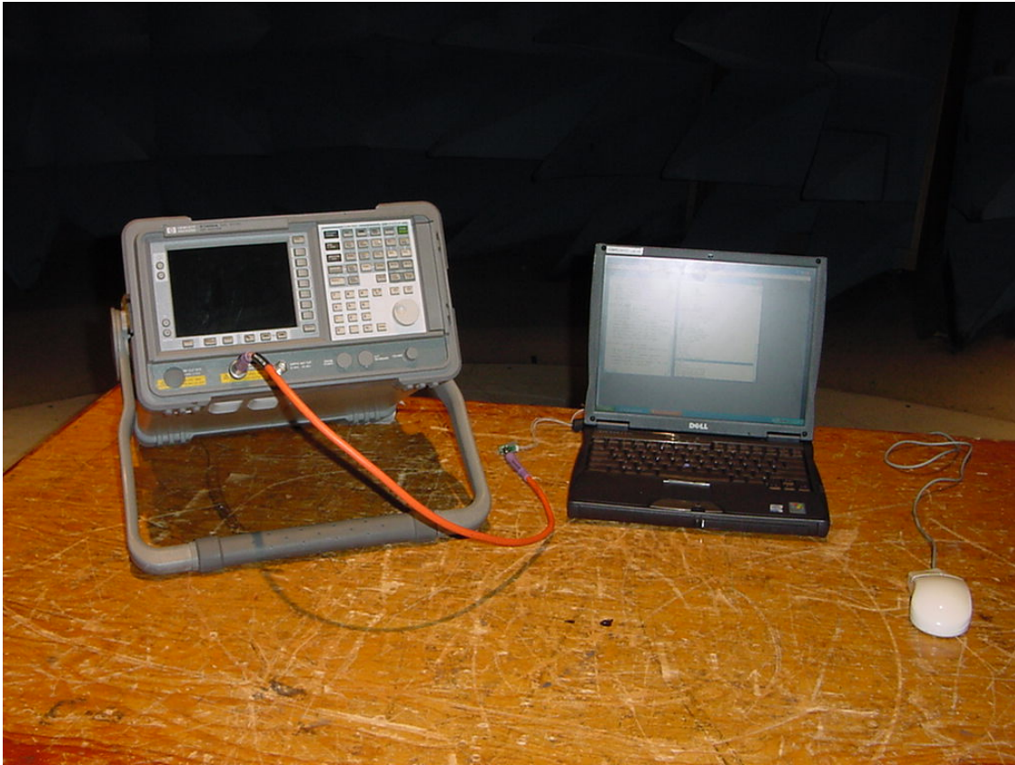
Photograph 6. Conducted Measurements Setup
