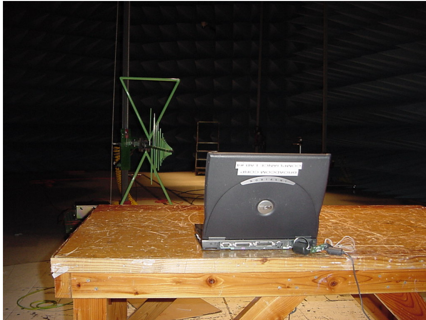
Photograph 2. Radiated Emission Test Setup 30-1000MHz
