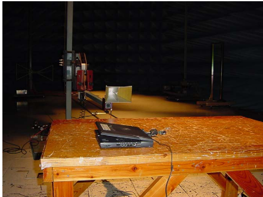
Photograph 3. Radiated Emission Test Setup 1-26GHz
