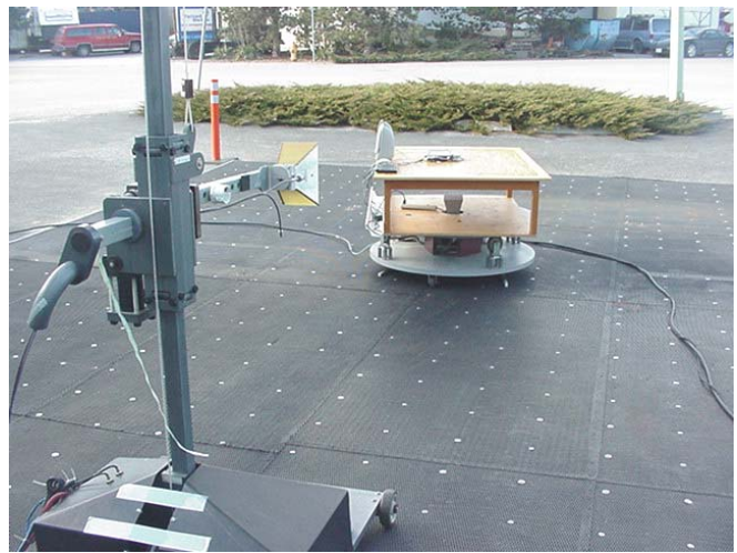
Photograph B.8-4 - Horn Substitution Setup
