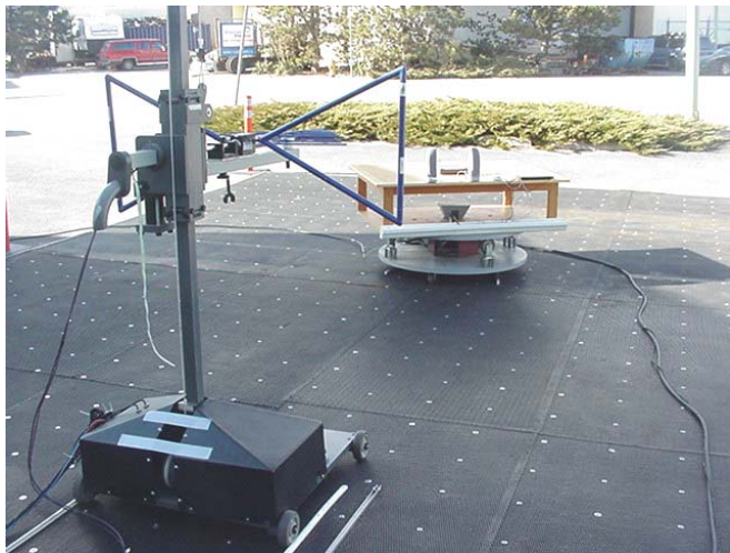
Photograph B.8-3 - Dipole Substitution Setup
