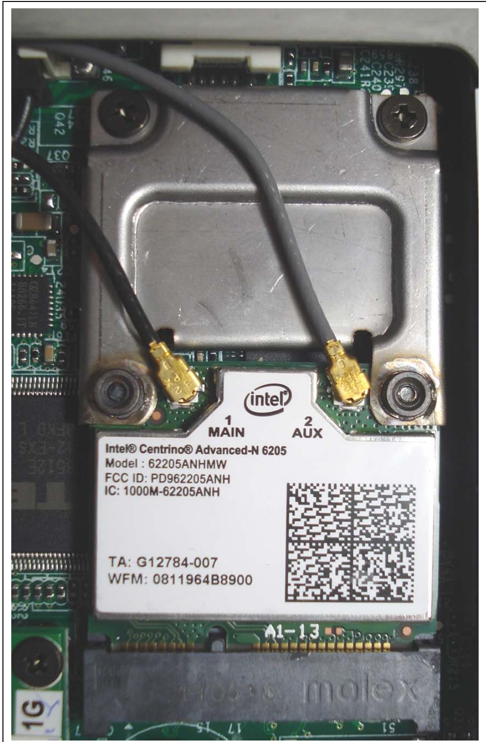
IX-62205ANH WLAN PCIe Half Mini Card installed in GD3080
