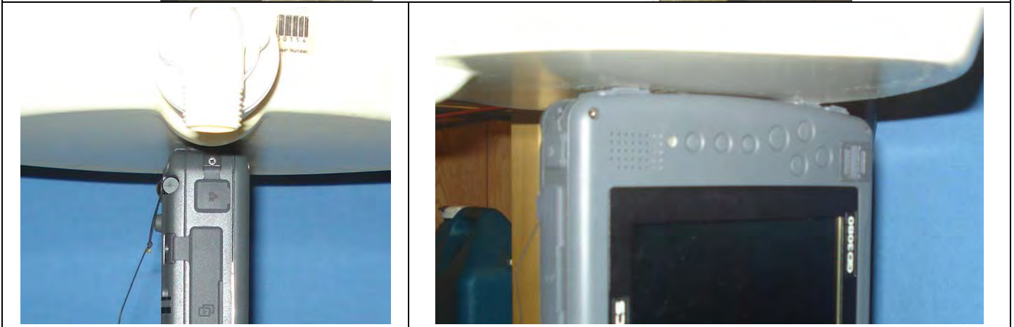
(“90° Portrait”) Adjacent Edge of DUT touching SAM phantom (planar section) – WLAN Main Antenna
