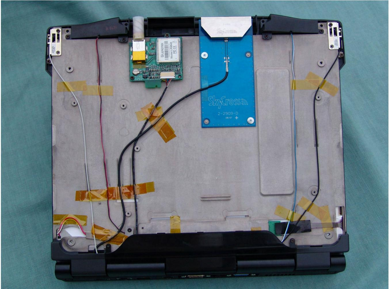
**WLAN Main and Aux antenna located upper right and left hand sides of display.**
