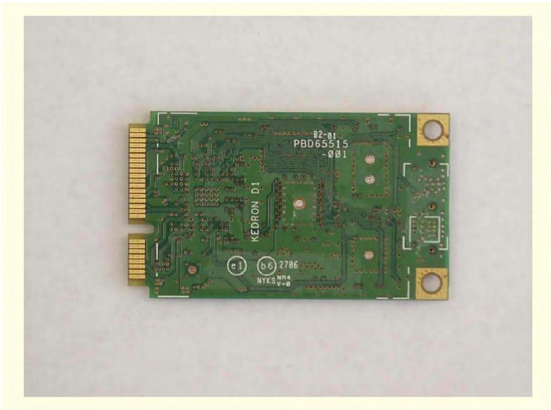
Top View of the IX-4965AGN Shielding Removed
