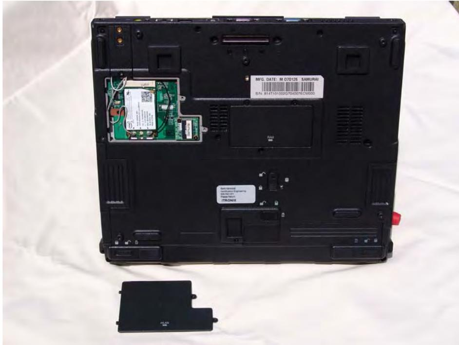
Enlargement of IX605 with KBCIX-4965AGN installed
