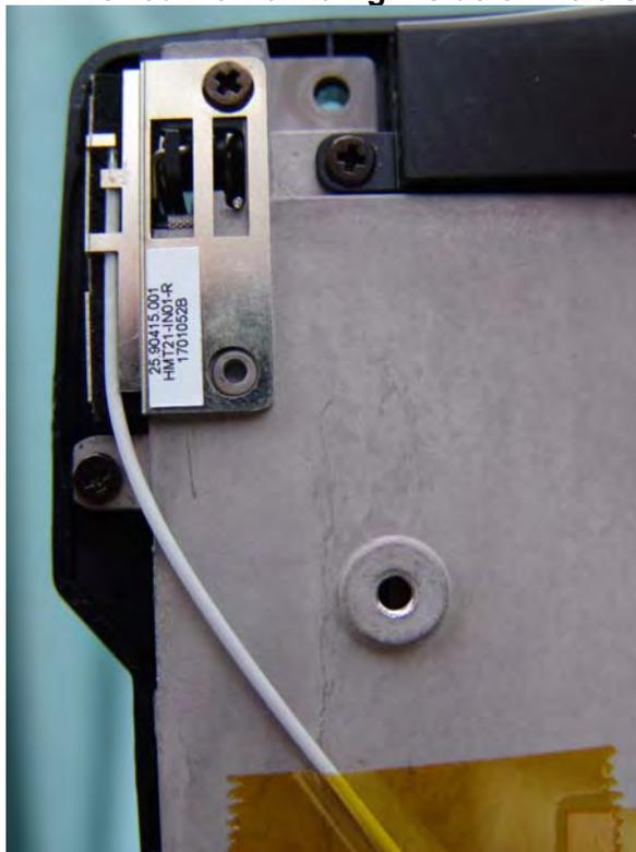
WLAN location bottom of the IX605, cover removed
