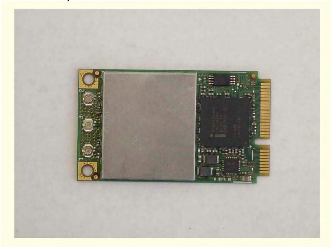
Bottom View of the IX-4965AGN Insulation Removed
