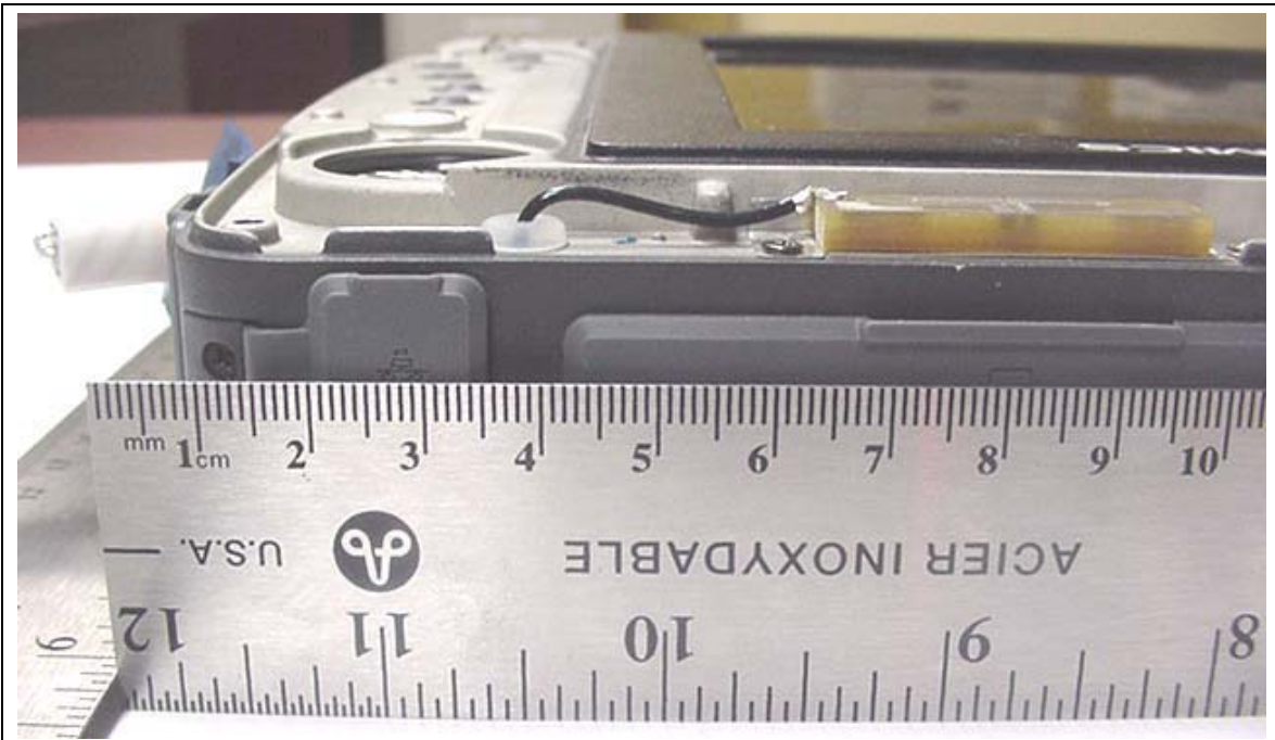
WLAN AUX Antenna Distance to Adjacent Edge (6.5 cm)
