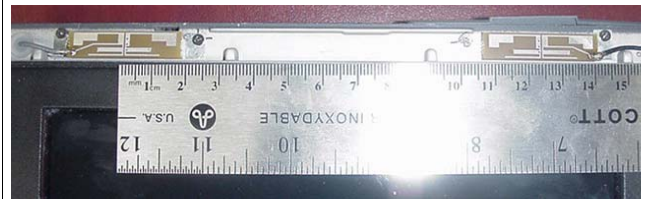
WLAN MAIN Antenna Distance to WLAN AUX Antenna (8.5 cm)
