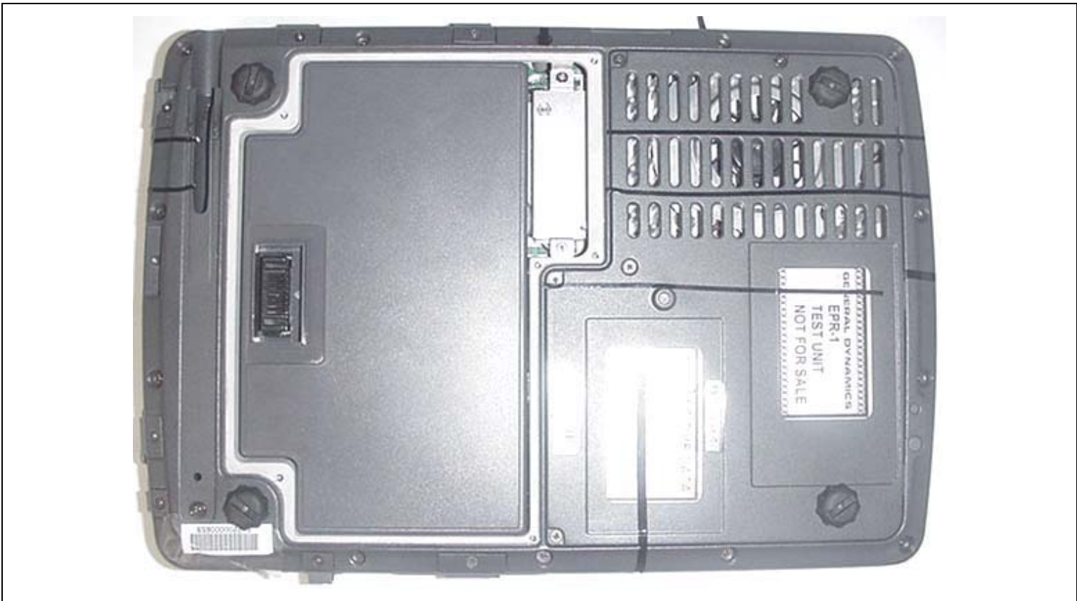
Bottom Side of Tablet PC with Battery Cover Removed
