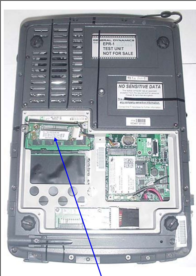
Bottom Side of Tablet PC (Battery Removed) with Bluetooth Cover Removed
