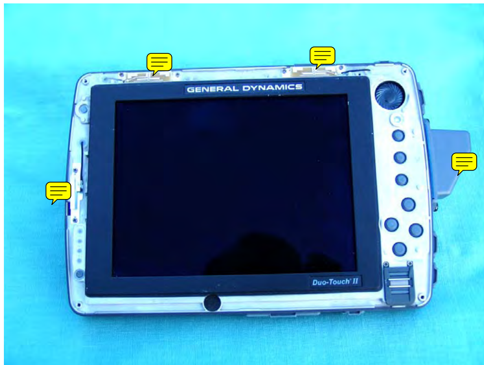
Bluetooth Antenna Left Side Center on IX350 Above, Shown Below_____
