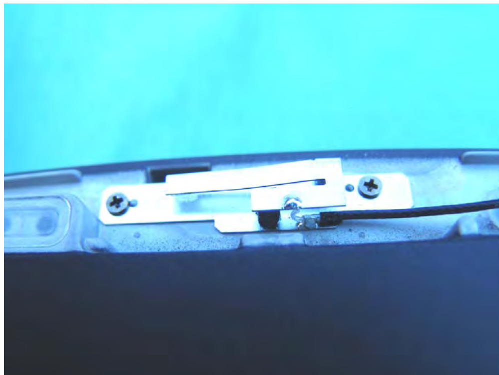
Bluetooth Antenna Left Side Center on IX350 Above, Shown Below_____
