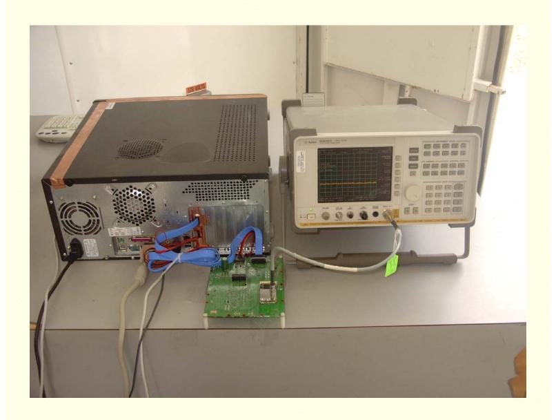
Conducted Emissions at Antenna Terminal Setup
