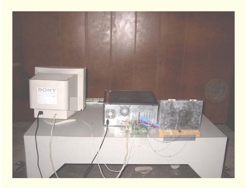
Radiated Emissions Measurement (Rear View) Setup
