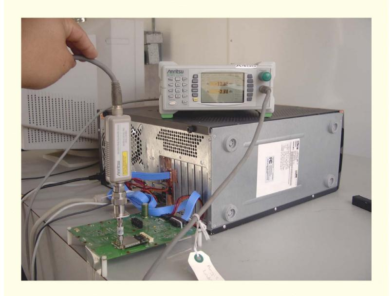
Maximum Peak Output Power Measurement Setup
