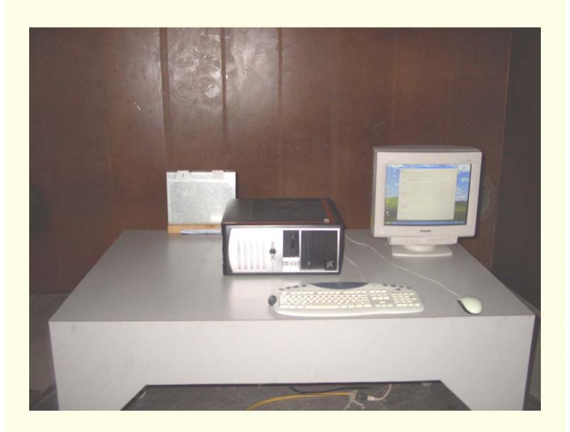
Radiated Emissions Measurement (Front View) Setup
