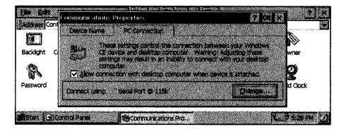
Tapping the change button will display a drop down list box from which you can select the required baud rate. The option 'Serial Port @ 115k' is the fastest available speed.
