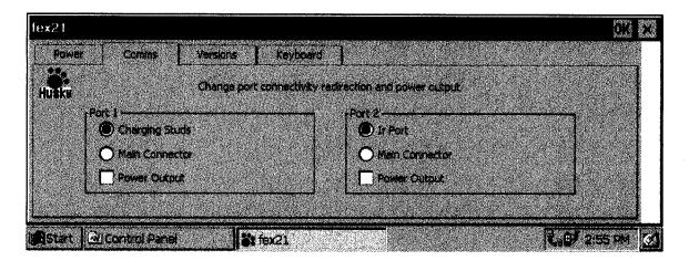
You will also notice that this screen also allows the user to redirect port two output in the same way. As the secondary COM port on the fex21 utilises com4 the IR port has to be disabled and redirected to main connector to allow 9-way comms.
