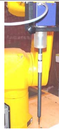
EX3DV4 E-Field Probe
