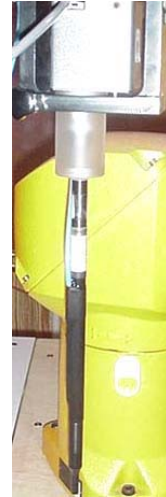
ET3DV6 E-Field Probe
