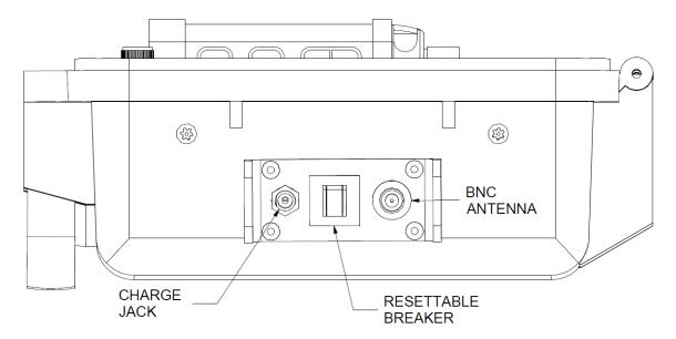
The antenna and charge jack are located on the right side of the receiver. The unit may be used while it is being charged.
