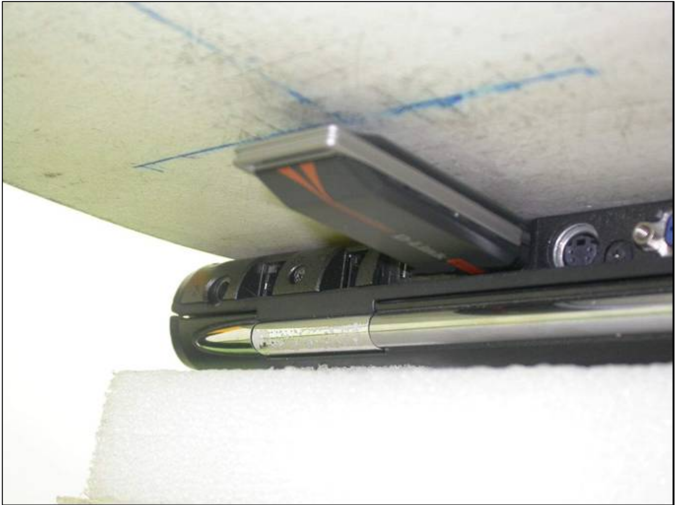
The bottom of the EUT to the flat phantom distance 7 mm
