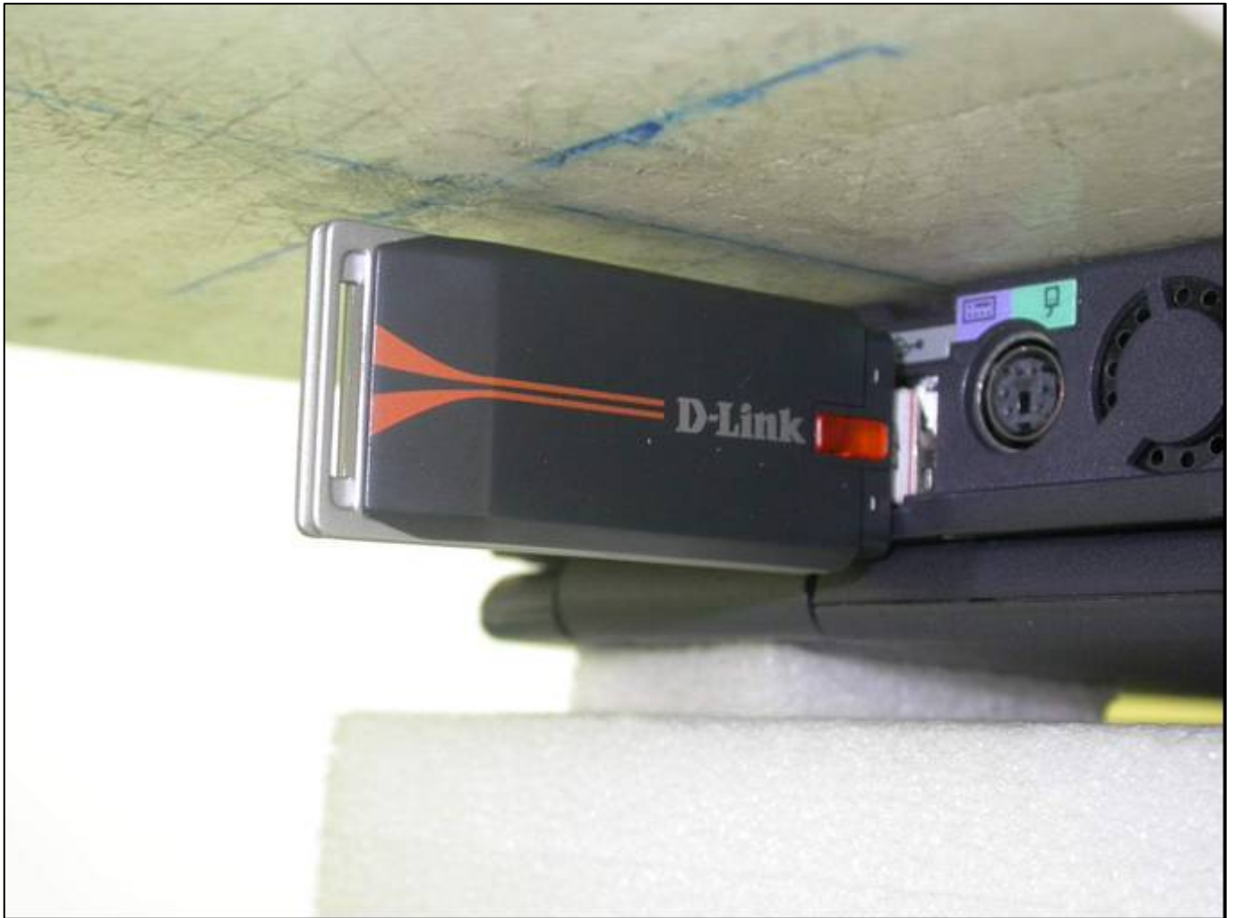
The edge of the EUT to the flat phantom distance 6 mm
