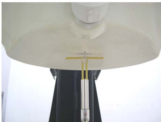
Fig 7.2 Photo of Dipole Setup
