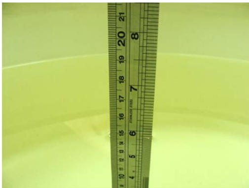
Fig 6.1 Photo of Liquid Height for Body SAR
