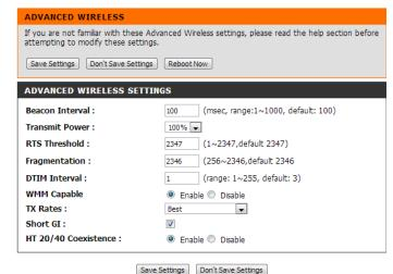
**Short GI:** Check this box to reduce the guard interval to 400 ns. This can increase the throughput rate provided that the delay spread of the connection is also low. However, it can also increase error rate in some installations, due to increased sensitivity to radio-frequency reflections. Select the option that works best for your installation.
