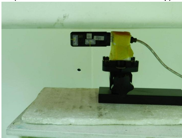
USB Cable Plug-in for USB Configuration 4 (Vertical Back with Phantom 5 mm Gap)
