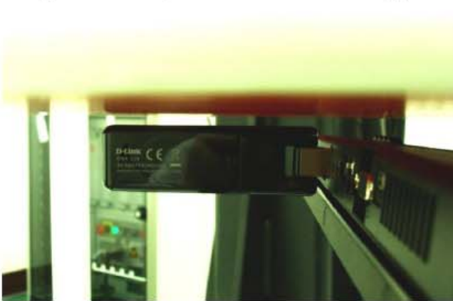
USB Cable Plug-in for USB Configuration 3 (Vertical Front with Phantom 5 mm Gap)
