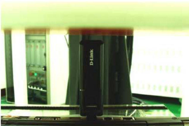
Direct Laptop Plug-in for USB Tip Mode (Tip Mode with Phantom 5 mm Gap)
