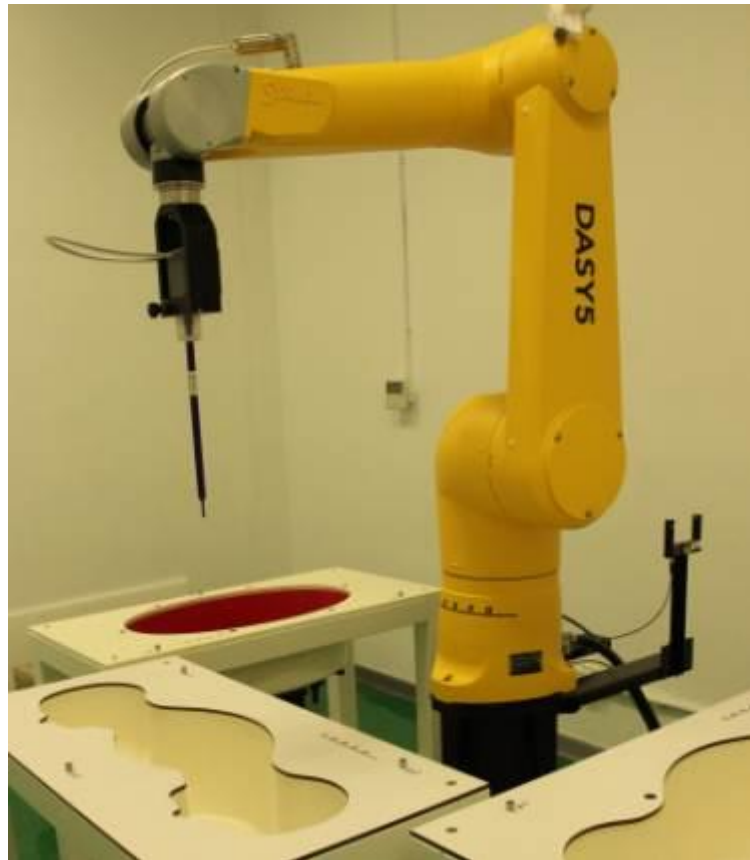
Picture D.6 DSY5 system Set-up
