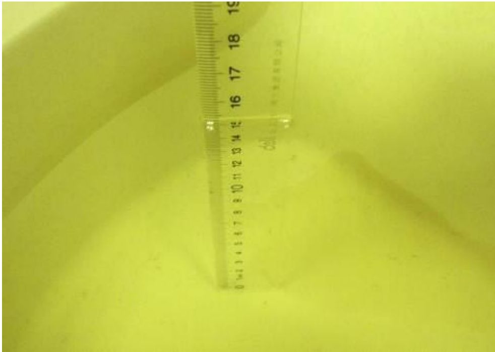
Picture 7-2: Liquid depth in the Flat Phantom (1900 MHz Body)
