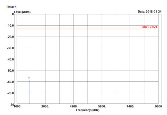
Site : 966 chamber 1 Condition: PART 22/24 Vertical Remark : LTE\_Band 5\_Link\_CH20600
