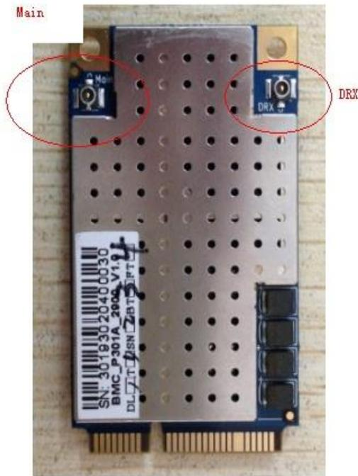
Figure 2-4 description of DWM-800B RF connectors
