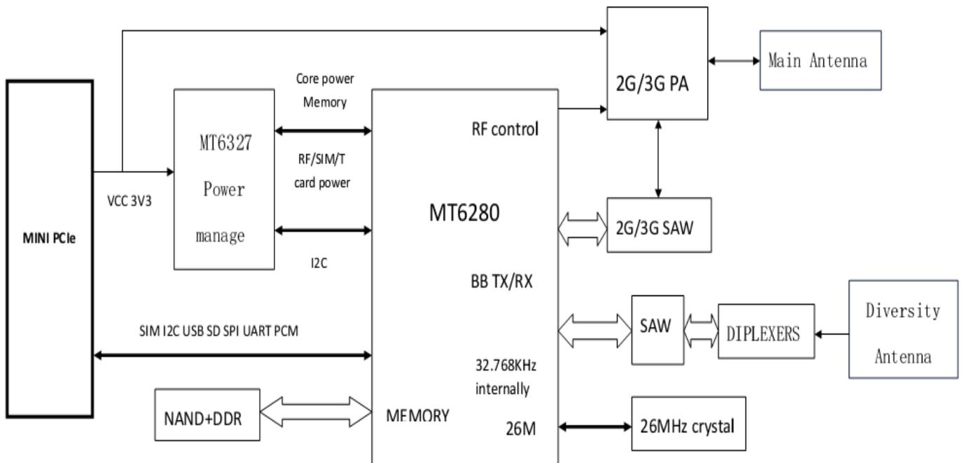
Figure1-1 DWM-800B block diagram
