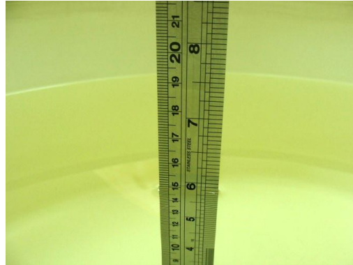
Fig 6.1 Photo of Liquid Height for Body SAR
