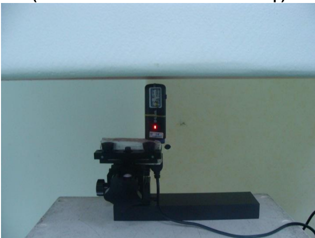
USB Cable Plug-in for USB Configuration 5 (Tip Mode with Phantom 5 mm Gap)
