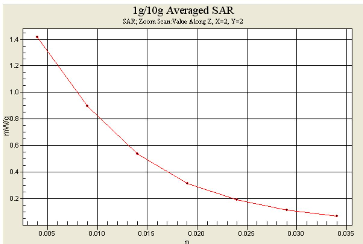
**#02 GSM1900\_GPRS8\_Horizontal Down\_0.5cm\_Ch661****DUT: 020329**
