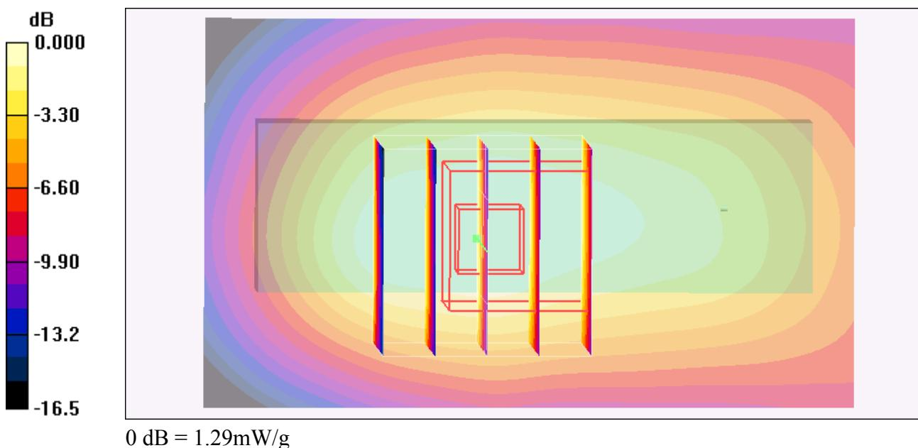
**#30 GSM850\_GPRS12\_Horizontal Up\_0.5cm\_Ch251\_2D****DUT: 020329**
