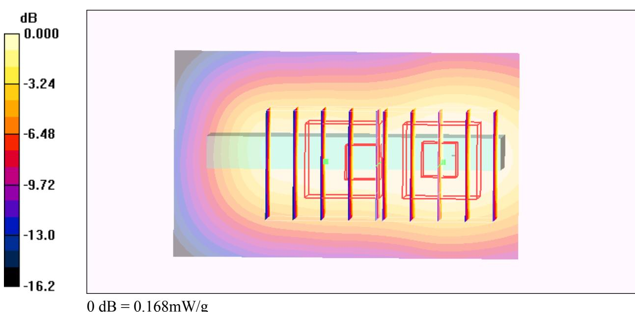
**#03 GSM1900\_GPRS8\_Vertical Back\_0.5cm\_Ch661****DUT: 020329**
