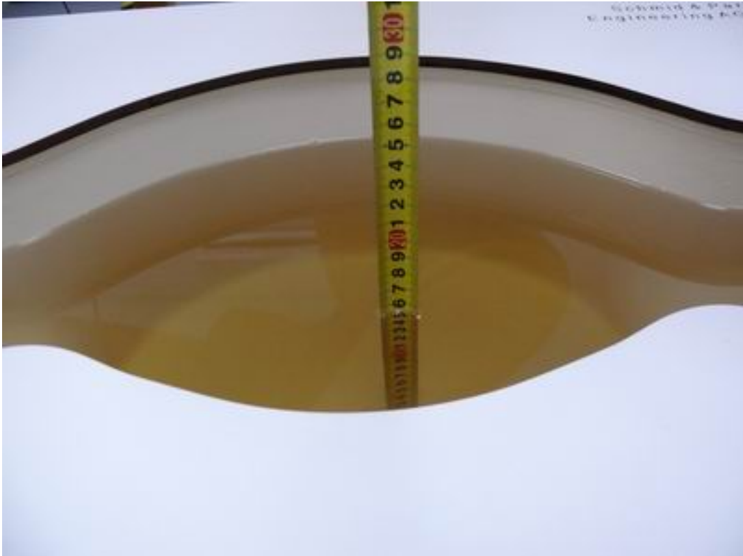
Picture 3: Liquid depth in the Flat Phantom (835 MHz) (15.4cm deep)
