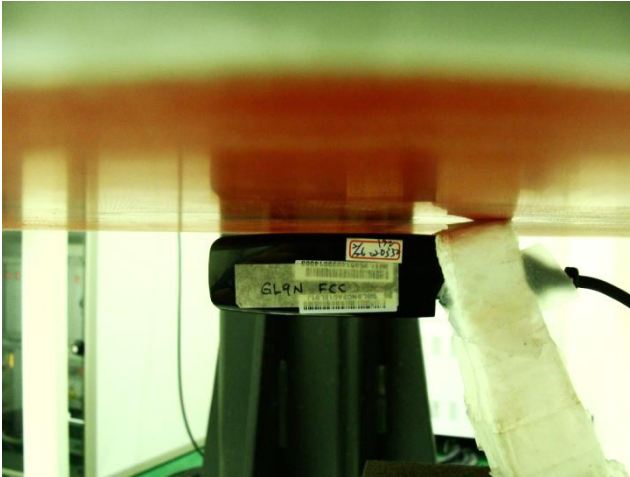
USB Cable Plug-in for USB Configuration 3 (Vertical Front with Phantom 5 mm Gap)
